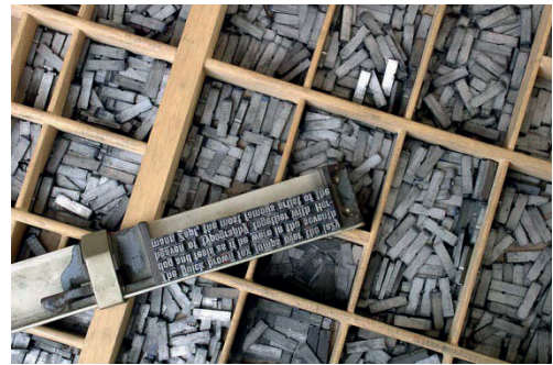
Movable type sorted in a letter case and loaded in a composing stick on top 1 .
