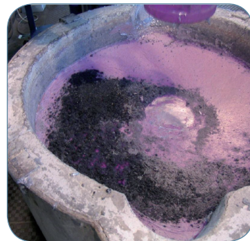
Fig. 4: After the MTS 1500 treatment is complete a dry dross remains, significantly reducing the Aluminium loss during treatment.
