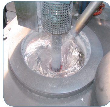
Fig. 2: The vortex has been formed and the flux is dispensed deep into the melt.
