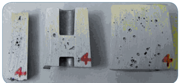
Fig. 15: Three sectioned bosses from the casting made after MTS 1500 treatment with 0.015% COVERAL MTS 1524 flux.
