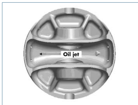
Fig. 10: Underside zone of the piston crown.
