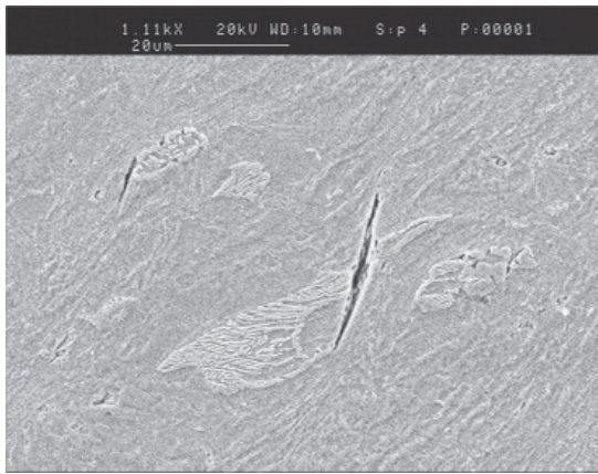
Fig. 9: SEM micrographs showing microstructural details of the ECAP pressed samples. (a) 1 pass; (b) 3 passes; (c and d) four passes.
