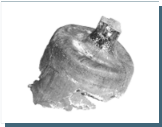
Fig. 2: An example of the not completely extruded material belonging to the last part of the billet.
