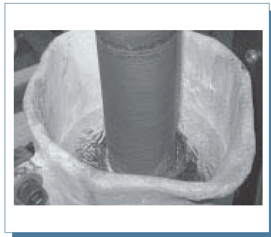
Fig. 6: Cooling of a 5 kg (11-pound) cup of melt.
