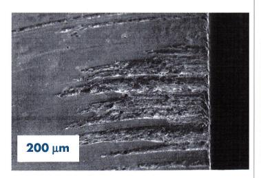
Figure 8: Typical damage on the lateral belt of the TiN coated cool forging tool. SEM micrograph of the surface near the transversal section; longitudinal axis of the punch: horizontal
