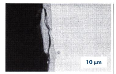
Figure 6: Partial scaling off of the CrC layer in a critical core pin. SEM micrograph pf a longitudinal section (the axis of the core pin is vertical)
