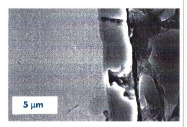
Figure 7: Typical features of an examined TiAIN coated core pin after a service life of 22000 shots. SEM micrograph of a longitudinal section (the axis of the core pin is vertical)
