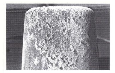
Figure 3: Surface features at the head of the CrC core pin in the most critical location after 10990 shots \_
