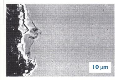
Figure 5: Typical features of CrN coated pins. SEM micrograph of a longitudinal section (the axis of the core pin is vertical)
