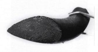
Fig. 7: Fracture surface of a spring failed in service
