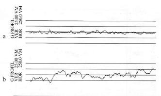
Fig. 6: Comparison of the surface roughness profiles of two shot peened springs. (a) conventional spring, RA= 1.85  $\mu$ m; (b) abnormally shot-peened spring, R<sub>A</sub>= 5.00  $\mu$ m
