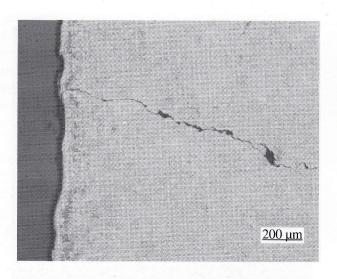
Fig. 8: Microcrack nucleated from a surface defect
