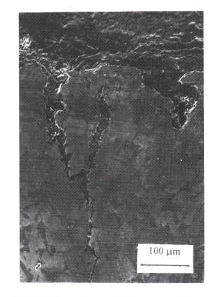
Fig. 11: Fracture surface of a broken roll axle
