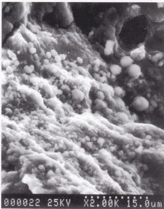
Fig. 12: Fretting deposits on crack surface of B-alloy
