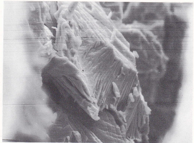
Fig. 11 - As per Fig. 10; crack tip; g = 1450 .
