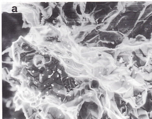
Fig. 7 - (a) as per Fig. 3, 20 h, 70°C; intergranular attack with barely marked fine parallel pleat pattern; g = 620 ; (b) as per Fig. 3, 90°C; intergranular attack with fine parallel pleat pattern; g = 920 .
