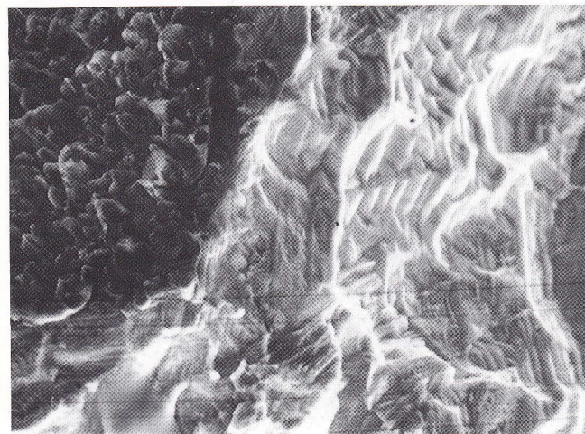
Fig. 8 - As per Fig. 5; transgranular trend of crack close to mechanical fracture region; g = 900 .
