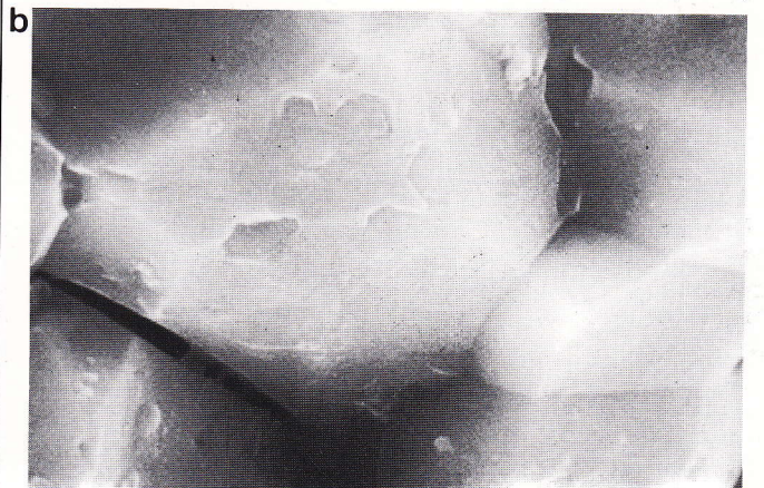
Fig. 7 - Appearance of surface fracture of the WZ. Dimples typical of ductile fracture are absent.
