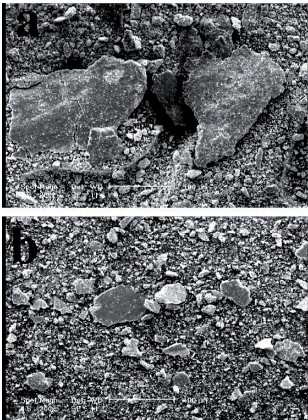
Fig. 6 - SEM micrograph of wear derbies of the heat treated samples under 60 N load and sliding velocity of 0.15 m/s: (a) QT and (b) DCT24.
