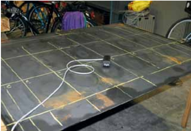
Fig. 4 - 8 mm EHS-Steel plate unannealed with the probe for the MikroMach
