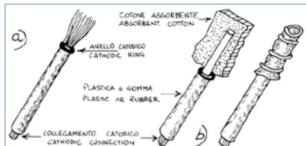
Fig. 1 – Instruments of electrochemical painting: a) brush; b) galvanic pad
