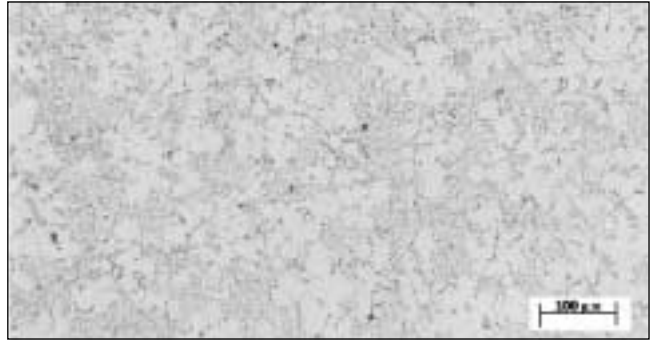
Fig. 1 – Microstructure of Direct Squeeze Casting samples. Material: AlSi8Cu3Fe + TiB 2 (6%wt.) particles.
