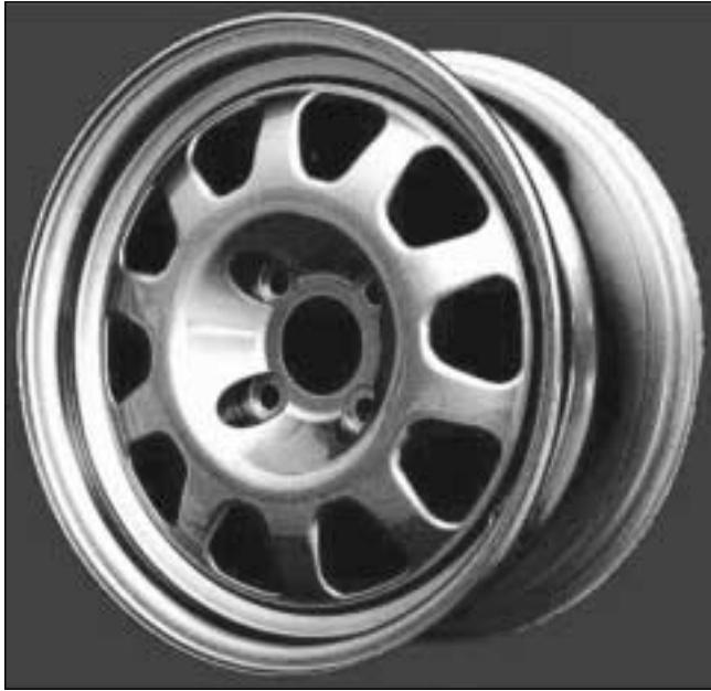
Fig. 1 – Demonstrator disc made of aluminium alloy welded onto an aluminium series 5000 rolled rim.
