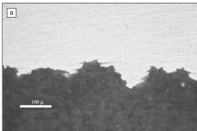
Fig. 5 – Stress corrosion cracking test in solution number 2, E_{corr} . Transversal secondary cracks.
