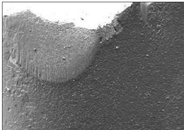
Fig. 10 – Flank wear nature of the CER2 type cermet with the TiN/(Ti,Al,Si)N/TiN coating ( f=0.1 mm/rev, a_p=1 mm, v_c=400 m/min).
