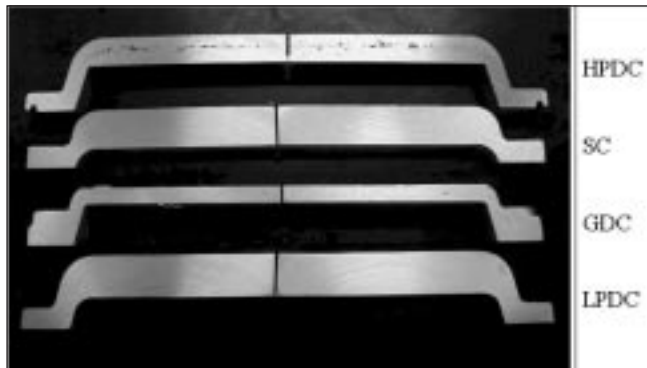
Fig. 9 – Macroscopic examinations of the covers after sectioning.
