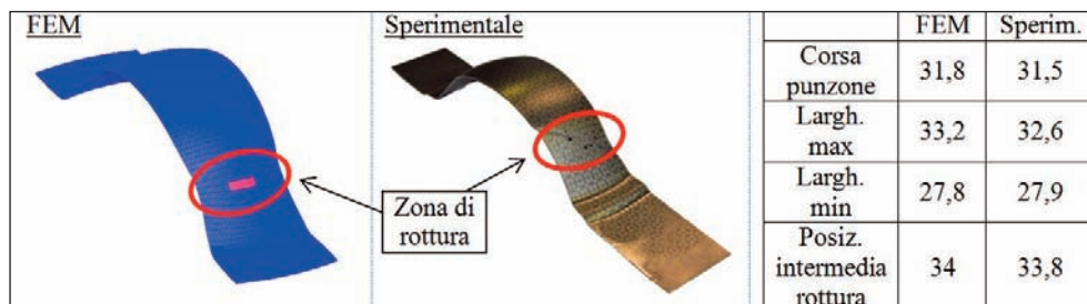
Comparison between FEM results and experimental deformations measured after Nakazima test at 20°C on 34 mm width sheet.
