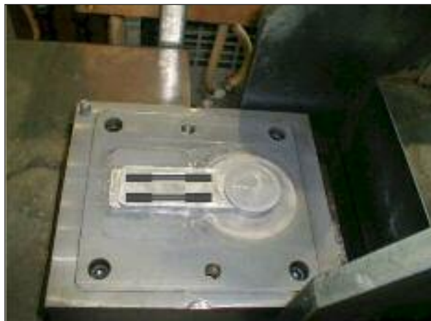
FIG. 3 Wide flat 'Finger-Die' arrangement used for thixoforming A201 parts for mechanical property evaluation.
