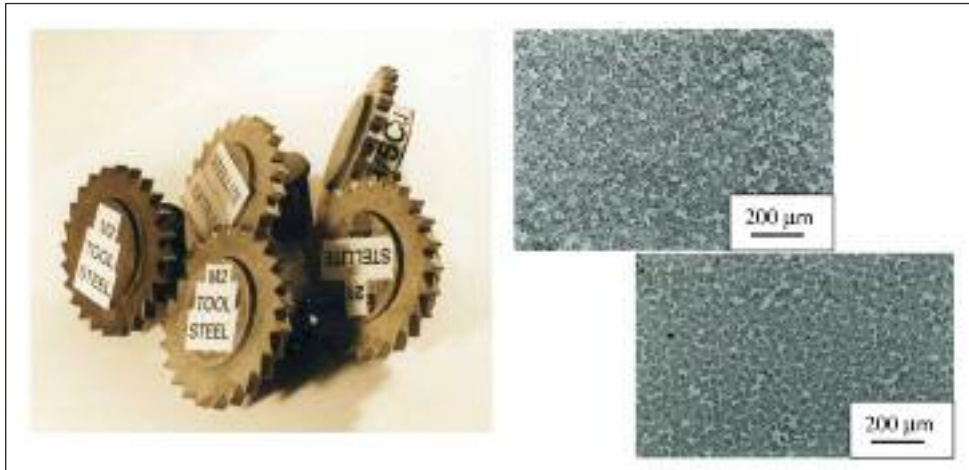
FIG. 8 Thixoformed M2 tool steel cog wheels and resulting typical microstructures: GFM feedstock (top) and Sprayformed feedstock (bottom). Other alloys are also shown in the picture.
