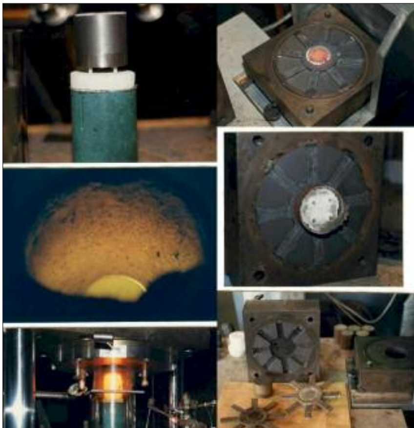
FIG. 3 Thixoforming sequence for M2 tool steel.
