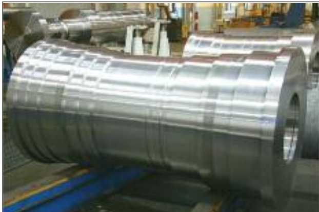
FIG. 19 Quality heat-treated and machined FB2 Forging; final weight 9,2 t.
