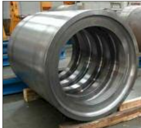
FIG. 7 Hollow shaft made of COST steel E, Boehler grade T505.
