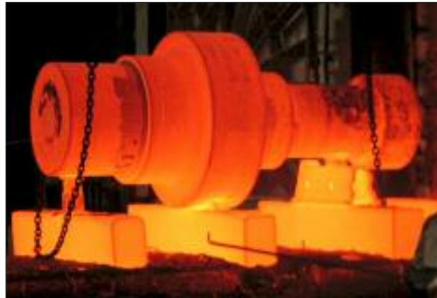
FIG. 14 Shaft component made of COST steel F, Boehler grade T507.
