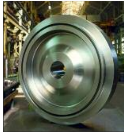
FIG. 2 Turbine disc made of 26 NiCrMoV 14 5 mod steel, Boehler grade V128SA.
