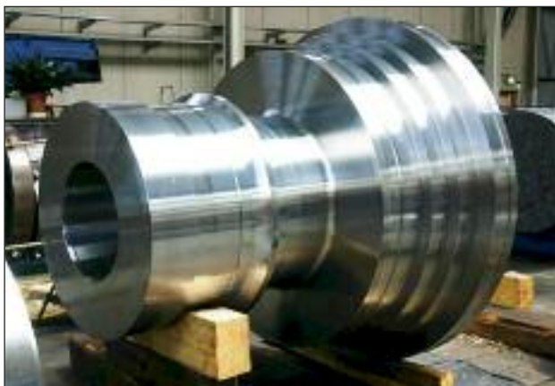
FIG. 13 Shaft component made of COST steel E, Boehler grade T505.
