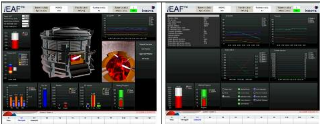
FIG. 1 iEAF® pagine operative del sistema. iEAF® SCADA operating displays.
