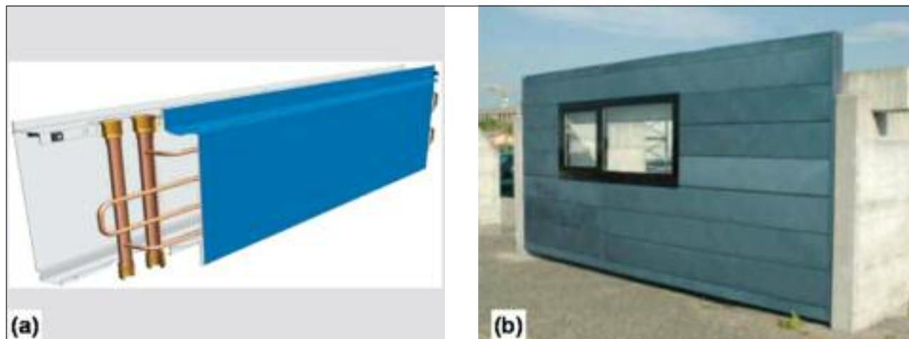
FIG. 6 Solabs®: (a) sketch of a facade element with solarthermic function (b) demonstration facade at EPFL Lausanne.
