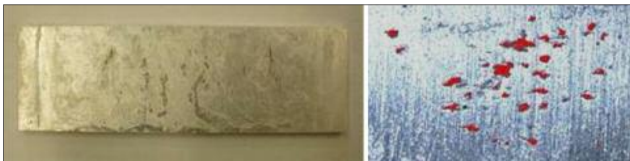
Fig. 5 Image analysis of a corroded surface.
