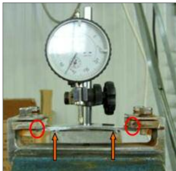
FIG. 2 Four point bending loading of the SCC samples.
