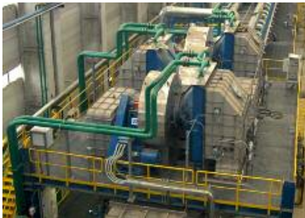
FIG. 7 Compact design for horizontal jet cooling.
