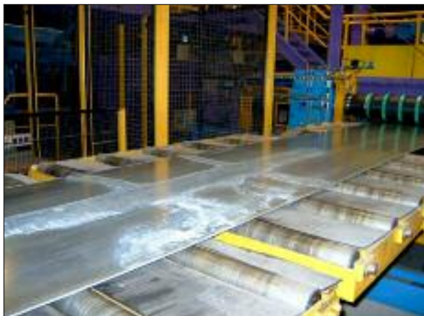
FIG. 2 Picture of white rust formation after long transportation and storage time.
