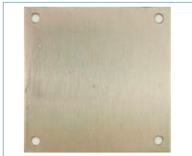
Figure 11: Stainless steel alloys after 18 months of deep sea immersion Sample size 100x100 mm a) 316 L SS; b) 2205 DSS.
