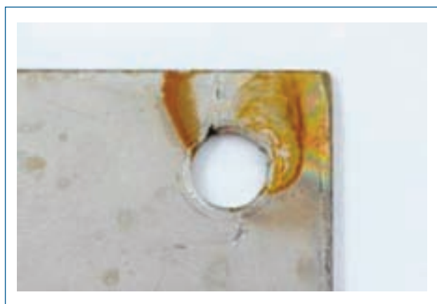
Figure 13: Crevice corrosion on sample 316 L SS after 12 months of deep sea immersion. Hole diameter: 6 mm.
