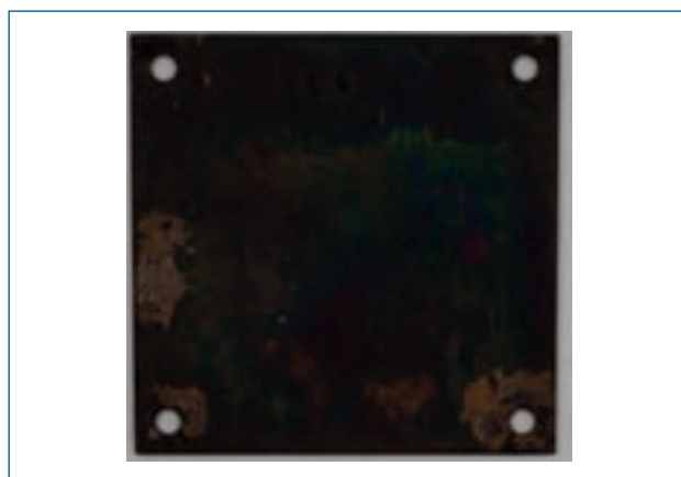
Figure 14: Cu-Ni 90/10 alloy after 18 months of deep sea immersion. Sample size 100x100 mm.
