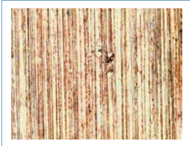
Figure 5: OM (100x) of AA 6082 before (a) and after 18 months of deep sea immersion (b).
