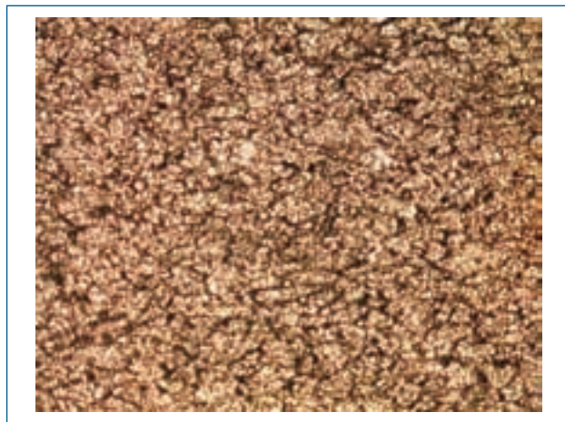
Figure 12: OM (100x) of the 316 L Stainless Steel before and after immersion 18 months of immersion.
