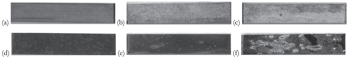
Figure 2: Typical photographs of AA2024-T3 pre-corroded tensile specimens exposed to the EXCO solution for (a)-(c) 2 h, 4 h and 24 h of EXCO solution and (d) – (f) 6 h, 168 h and 720 h of 3.5 wt. % NaCl solution, respectively.
