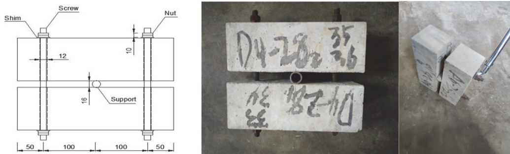
Figure 2: Long-term bending-load device
