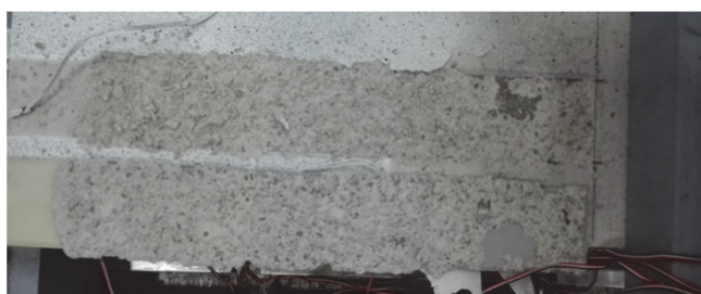
Figure 7: Debonding failure mode.
