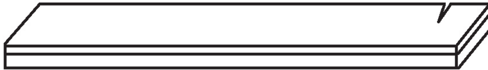
Figure 2: Schematic representation of the two-layered specimen.
