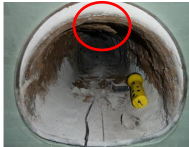
Figure 21: Failure in the model overload test.
