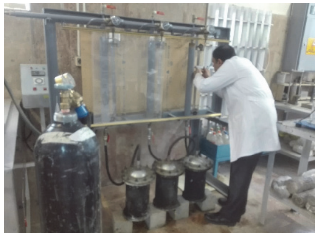
Figure 4: Hydraulic conductivity of the concrete test machine
