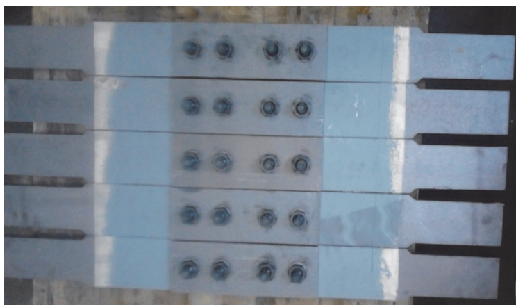
Figure 11: Blasted and half-coated specimens.
