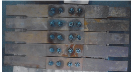
Figure 6: Blasted and rusted specimens.
