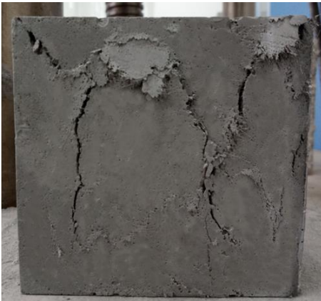
Figure 1: Failure mode of test specimens.
