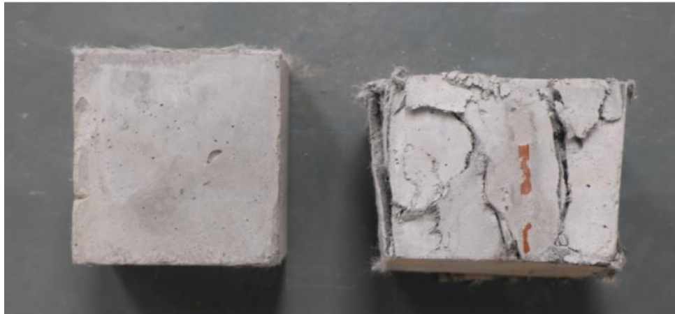
Figure 7: Failure mode comparison of ECC cube specimens in different phases of loading.
