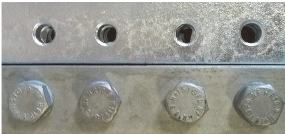
Figure 3: Comparison between specimens before and after sweep blasting.
