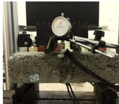
Figure 3: Installation Drawing of Modulus Test
