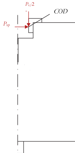
Figure 2: Detail of boundary conditions, see the half of specimen and the load application ( P_{sp} and P_v/2 ) with crack opening displacement ( COD ), position at load line.
