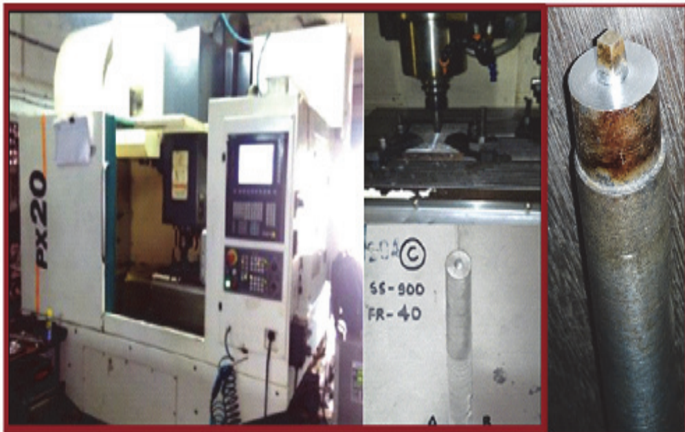
Figure 2: Friction stir welding on VMC machine with FSW joint.
