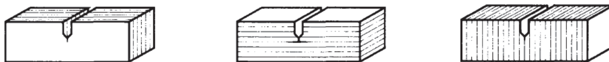
(a) L-T and T-L orientation: crack divider. (b) T-S and L-S orientation: crack arrester. (c) S-L and S-T orientation: crack splitting.
