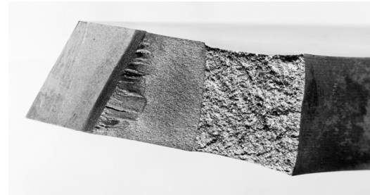
Figure 8: Twist crack fracture surface of mild steel angle notch test piece, fatigue loading.
