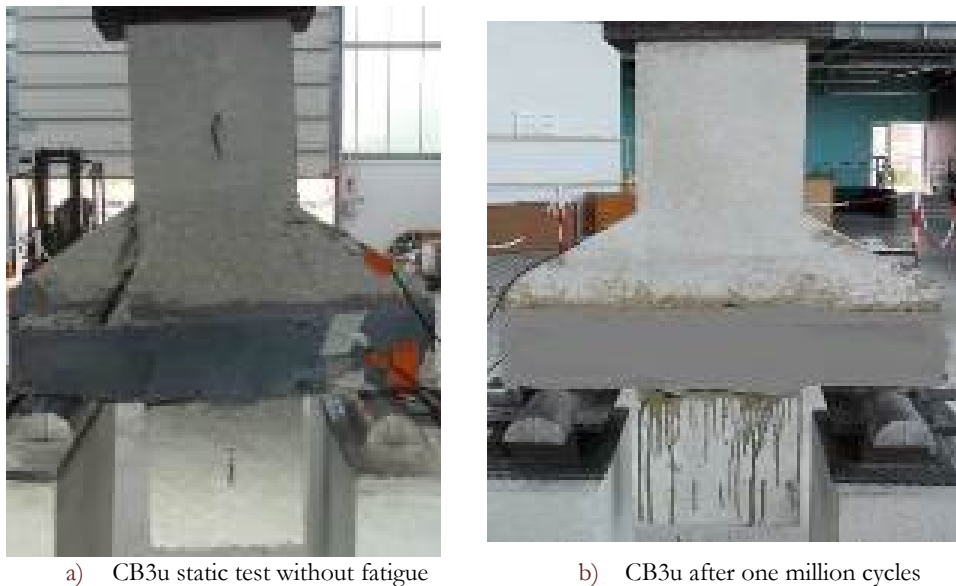
Figure 8: Cracking and failure in strengthened concrete corbel. a) CB3u-static loading to failure, b) CB3u -after one million cycles.
