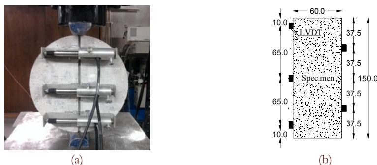
Figure 2: Geometry of the specimen and setup of the splitting tensile test (dimensions are in mm): (a) specimen front view (top of the panel), (b) specimen lateral view.
