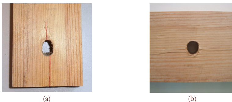
Figure 5: Failure modes of the T-connection: (a) failure at the centre member; (b) splitting at the side members.
