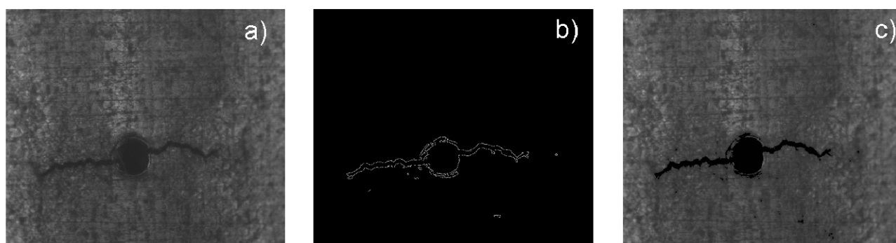
Figure 6: Image of sample S1 at maximum strain after applying 800 cycles. a) Raw image, b) image of the crack detected with the algorithm and c) detected crack superimposed on original image. The diameter of the hole is 150 \mu\text{m} .
