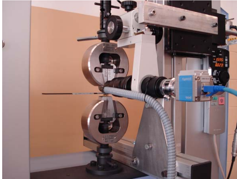
Figure 3: DBC test apparatus with CCD camera video image.
