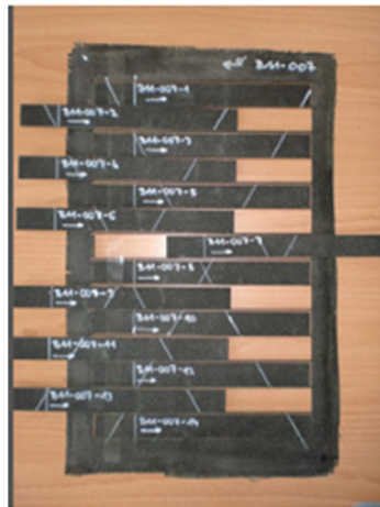
Figure 2: Typical composite plate after cutting using water jet in order to produce tensile test samples.
