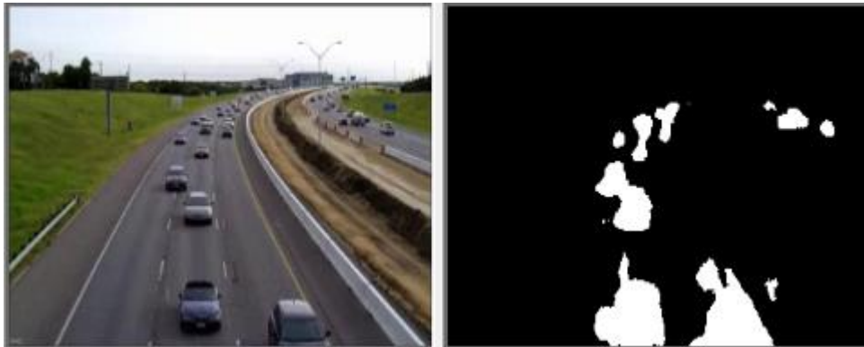
Figure 20: Motion based vehicle detection from CCTV footage
